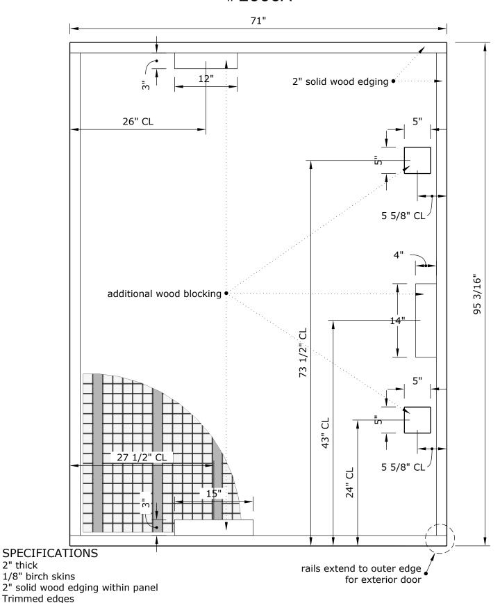
Premium grade torsion box core, medium grid with composite stiffeners
